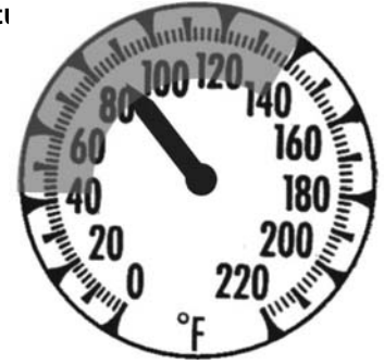
Danger Zone 41°F - 140°F
